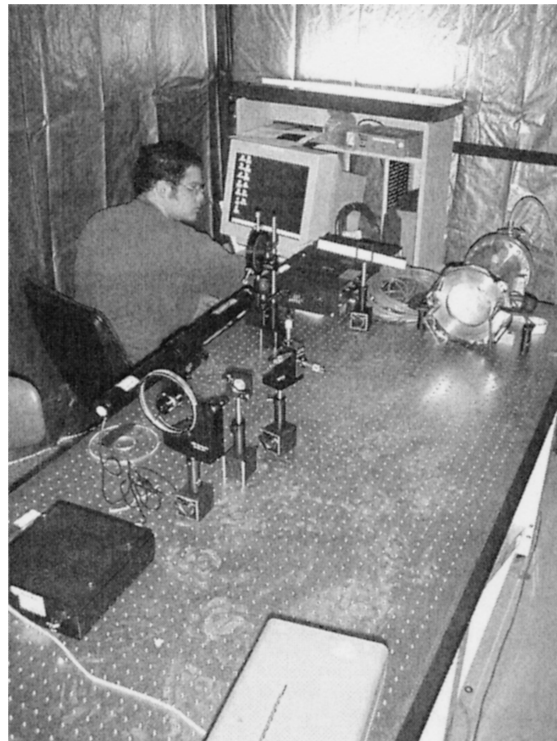
Fig. 2 Membrane inflation and interferometry test setup.
